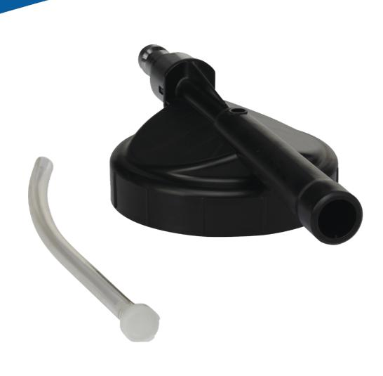
Foam Injector for foam cleaning. Water and chemicals are always mixed in the correct dosage from 0.40 to 10% and are foamed on the surface. Fits both large and small containers. Suction hose and filter provided.
