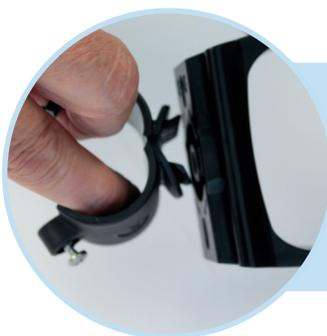
Keep the tool clamp open and insert the "wings" on the back of the clamp into the matching holes on the mounting piece.
